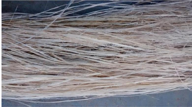
FIGURE 1: DRIED AND SORTED BANANA FIBRE
