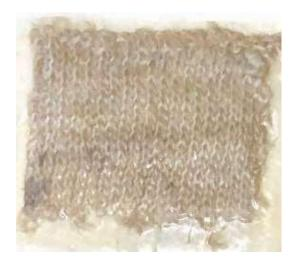
Plate 2. Jute:Acrylic (30:70) fibre
