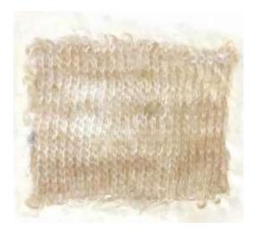
Plate 1. Jute:Acrylic (20:80) fibre
