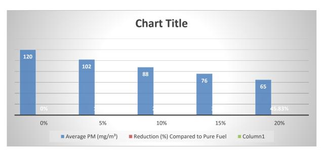
**Interpretation**: The results show a consistent decline in particulate emissions with increased water content, reaching nearly 46% reduction at a 20% water-in-fuel ratio.
